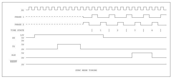
Figure 18. Sync Mode Timing
