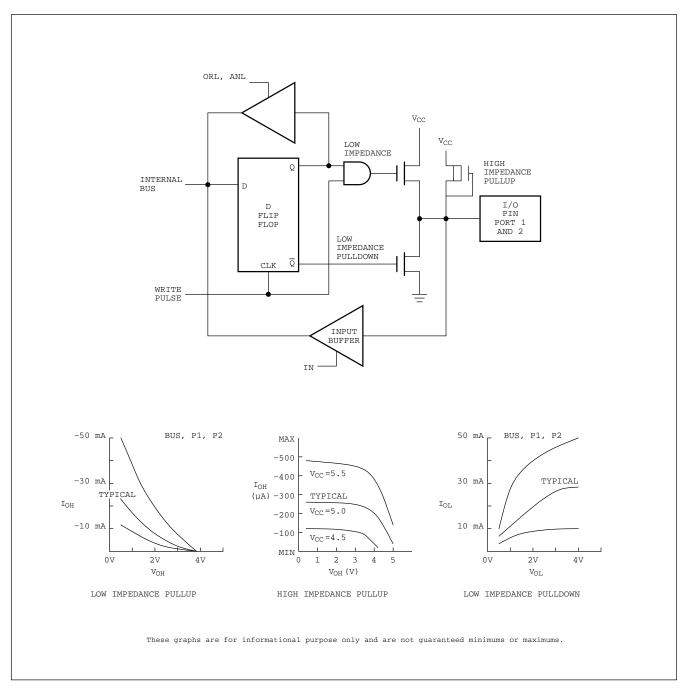
Figure 7. "Quasi-bidirectional" Port Structure
