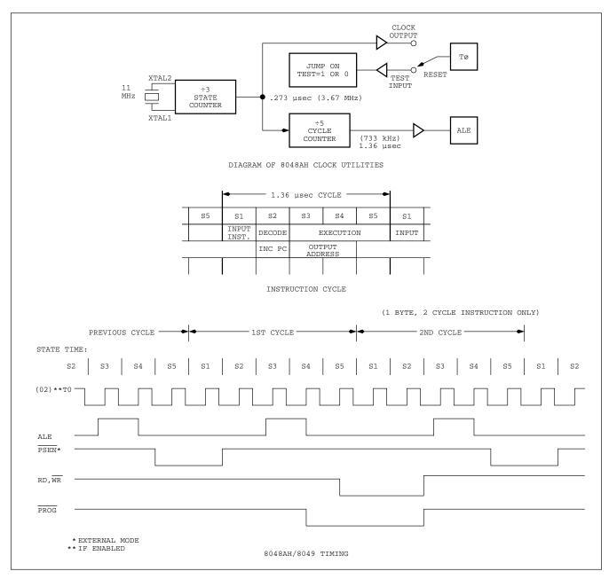
Figure 13. MCS-48 Timing Generation and Cycle Timing
