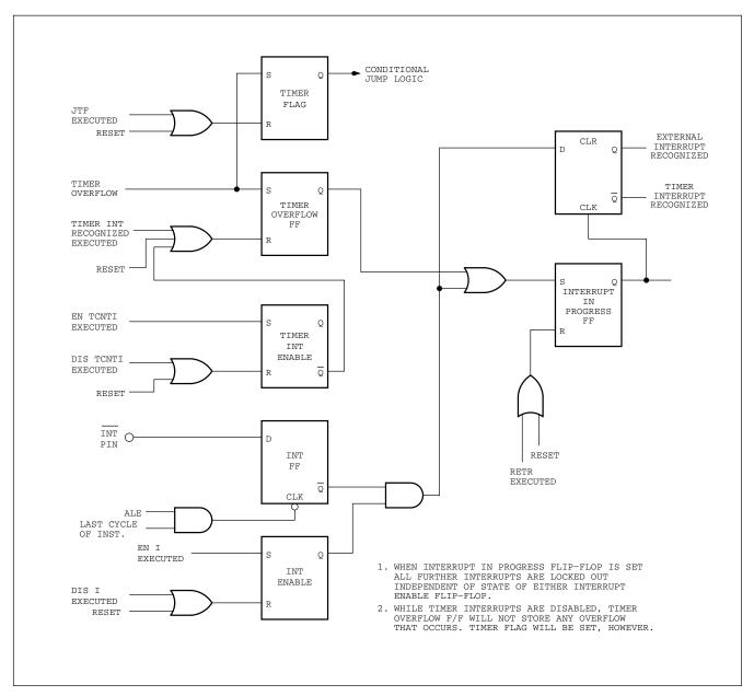
Figure 11. Interrupt Logic
