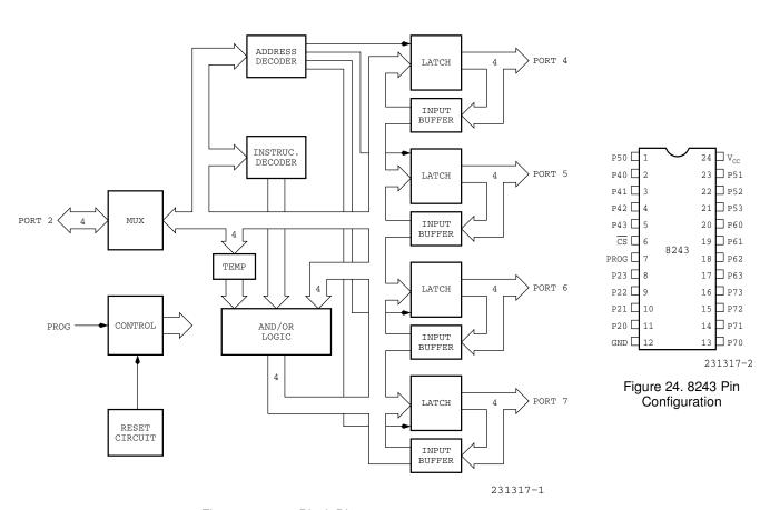
Figure 23. 8243 Block Diagram
