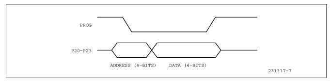
Figure 27. Output Expander Timing
