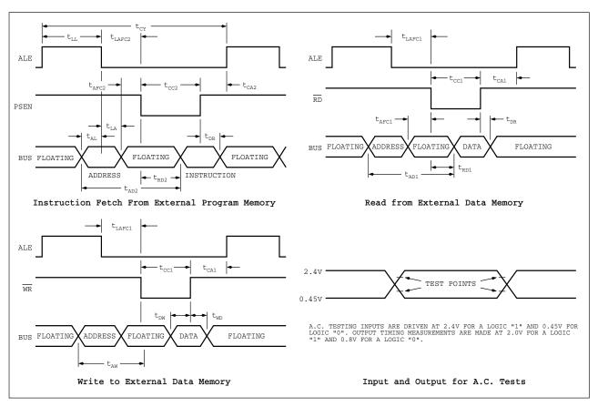
Figure 21. External Access Timing Waveforms
