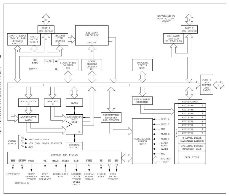
Figure 4: 8748H/8048H/8749AH/8050AH Block Diagram
