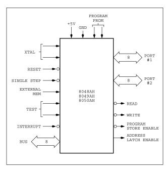
Figure 19. 8048AH and 8049AH Logic Symbol
