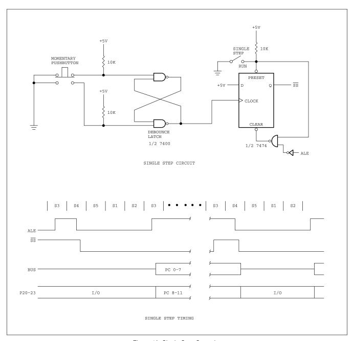
Figure 16. Single Step Operation
